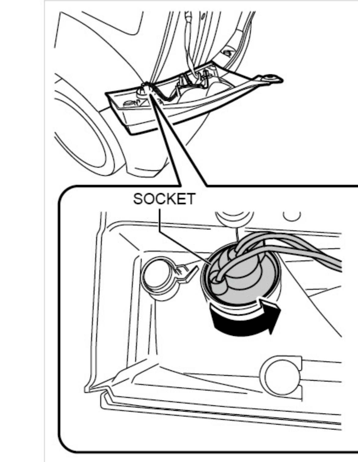
3. Move the socket in the direction of the arrow and remove the socket from the tail lamp.
