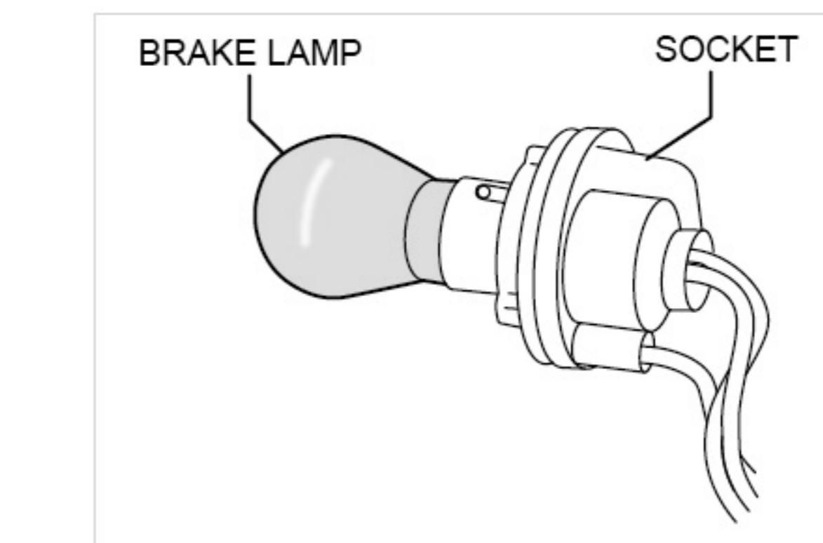
4. Remove the brake lamp from the socket.
